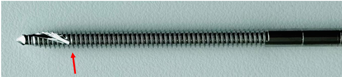
Figure 11: Full thread of drill pin (red arrow points to the first full thread)
