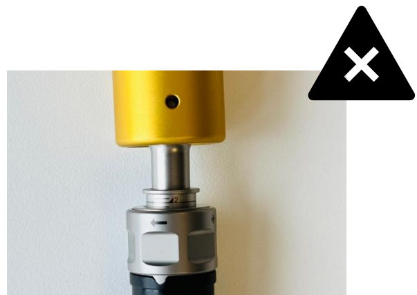
Figure 6 Incorrect position of the metallic hex thumb screw
